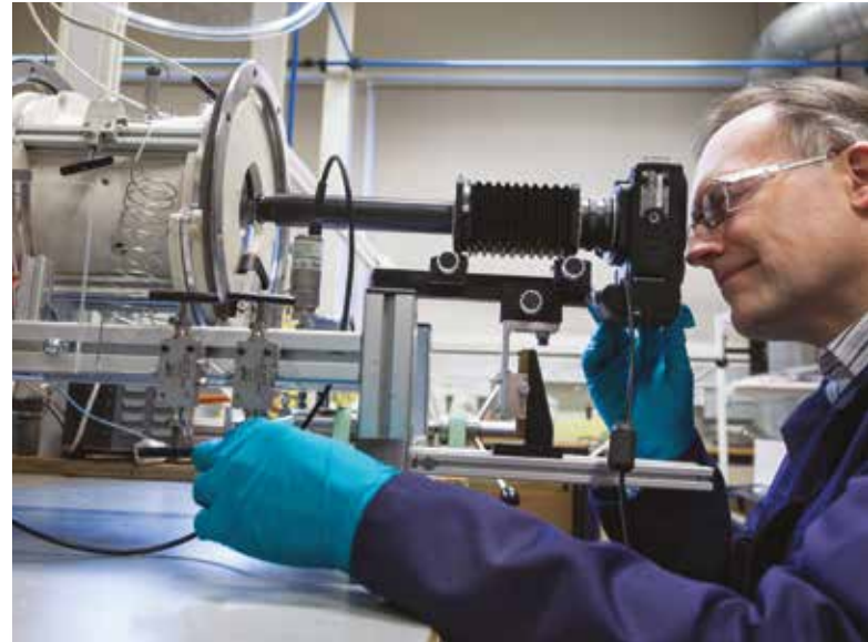
High pressure cell for measuring interfacial tension. Photo: SINTEF/Thor Nielsen
