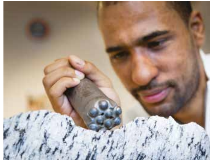
Developing drilling tools for hard rocks. Photo: SINTEF/Thor Nielsen
