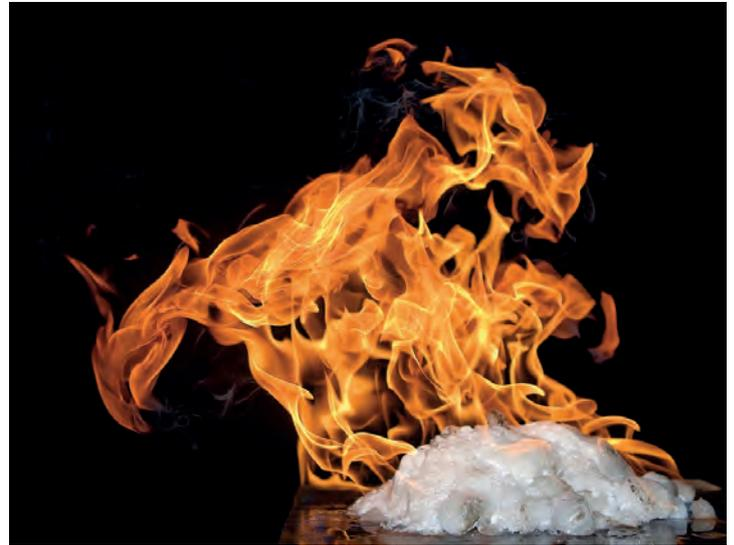
*Gas hydrates are one of the most important Flow Assurance challenges which depends on the chemistry of the system. Photo: Geir Mogen*
